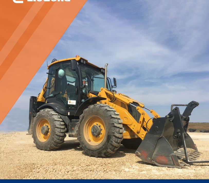
EnginePerkins1104D-44TAGross Power74.5 kW (100 hp / 101 ps) @ 2,200 rpmNet Power72 kW (97 hp / 98 ps) @ 2,200 rpmMaximum Speed41 km/hStandard Loader Bucket Capacity1.1 m³Backhoe Bucket Capacity0.2 m³Operating Weight9,480 kg
